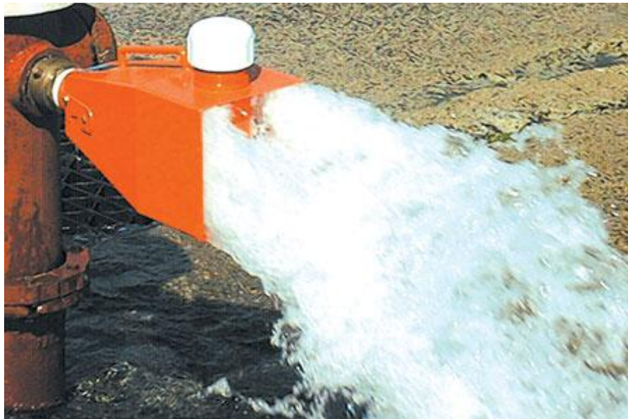
Figure 4-1 Diffuser Mounted Dechlorination Feed
